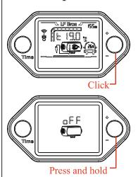
1.Click the Power Knob in the shutdown state, the screen lights up, the buzzer sounds once (release the button) and the heater is turned on.
