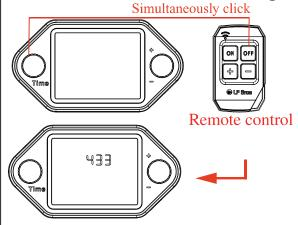
In the shutdown state, press and hold the TIME Knob of the control switch and the "OFF" key of the remote control at the same time.
